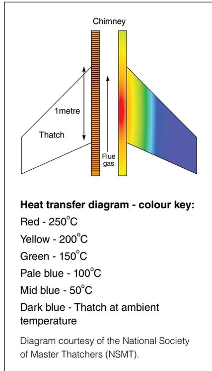
Over a period of time the temperature of the thatch chimney interface can become critical (approx. 200°C) and lead to a chain of events that cause a thatch fire.
